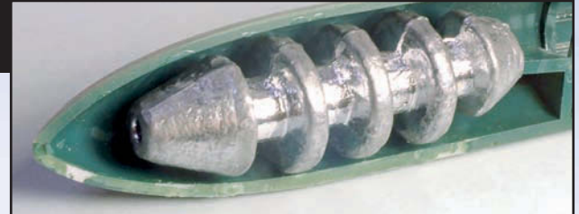
I found a fishing line weight with a perfect fit to the fuselage providing a good balance to the finished model.
