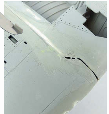
Fitting the Aires wheel bays distorted the shape of the mating surfaces between the centre and outer wing sections, requiring much work to fix.
