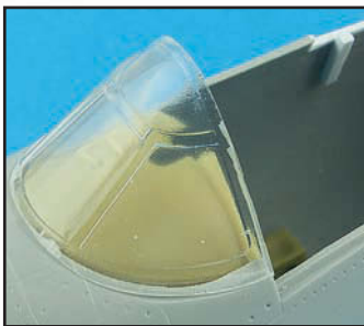
And checked for fit; the gap around the edges is neatly hidden by the windscreen framing!
