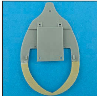
I spliced the Montex upper and Verlinden lower parts to create a new rear cockpit bulkhead.
