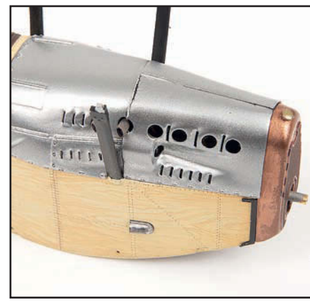
The last piece of cowling was glued in place and treated with hot air to get it to conform better. A new hinge will be constructed and the exhaust pipes refitted.
