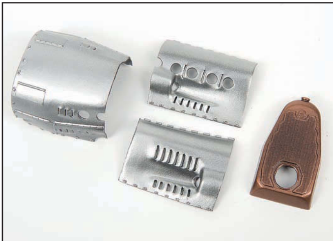
The radiator and canopy parts were primed in Mission Models Gloss Black before being painted with Alclad Aluminium and Copper respectively. The Aluminium cowlings were then treated with AK Interactive True Metal Aluminium paste and polished up.
