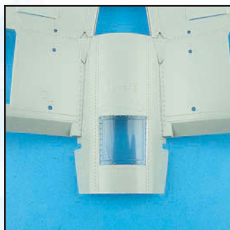
A section needs to be removed to allow for the clear resin window to be fitted.
