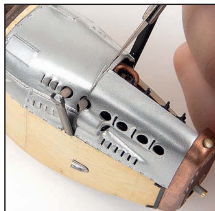
Test fitting the final cowling showed a small misalignment so I carefully trimmed the offending piece in situ.
